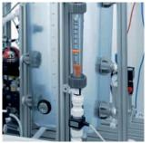
At a constant **flow rate**, the three input materials are mixed into a recipe on the Mixing station. The flow rate is recorded by an electronic flow sensor with an impeller, and is additionally displayed with a float-type flow meter. The controller sets the required flow rate by way of the analogue controlled pump.
