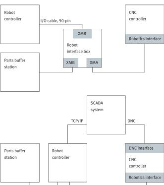
Level 1: Automated buffer operation via I/O communication between robot and CNC machine
