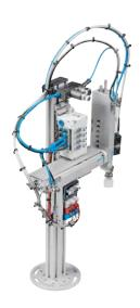
The Pick&Place module is a universal, 2-axis handling device for Pick&Place tasks. The position of the end-position switches, as well as mounting position and height, can be adjusted on this module. The module is supplied complete with vacuum generator, pressure switch, vacuum filter and suction gripper, valve terminal, pressure limiter and electrical interface. In another version, a parallel gripper is used instead of vacuum technology.
