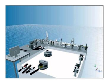
Robotino® SIM Professional is an ideal virtual learning environment for working with Robotino®. Identifying differences based on actual behaviour is the key to grasping, analysing and understanding new physical and technical phenomena. The software enables you to create any virtual 3D working environments for Robotino® and then to simulate the program created. The software is available in four languages (de/en/es/fr) and the language selection can be changed online.
