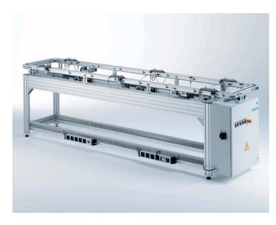
The material flow within the AFB lines is implemented by the pallet transport system. The six-packs are conveyed to the individual stations on pallets which are equipped with an identification system. The transport system features 4 stop points, and can be expanded at any time.
