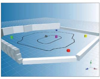
Robotino® SIM is a Windows software program for the 3D simulation of Robotino® in an exciting, predefined virtual experimentation environment.
