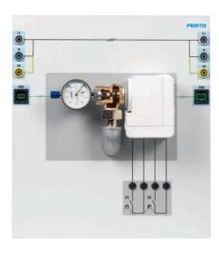
The heating actuator controls the heating water circuits in heating systems. The interior of the valve is visible, and an integrated gauge shows the stroke of the plunger. The valve is supplied entirely via the KNX bus. Two binary inputs are available as presence and/or window contacts and can be controlled via switches or external signals. The plate also contains the KNX system distributor for 230 V.
