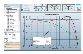
The convenient and intuitive **Drive-Lab** software supports the automatic recording of machine characteristic curves, the parameterisation of a static load and the simulation of load models for the examination of drives under realistic conditions. The comparison and optimisation of different drive concepts can be carried out in the form of project exercises. Sample configurations provide a quick and easy-to-understand introduction.
