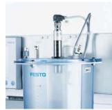
In the Filling station the **level** of the dosing tank is recorded with an analogue level sensor. By way of the continuously controllable pump the controller regulates the level to the appropriate nominal value. During filling, the level in the dosing tank is kept constant, thereby optimising the filling quality.
