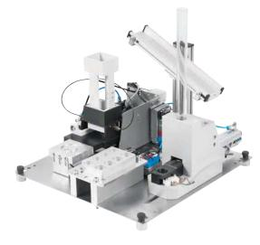
The robot assembly module is used to mount assemblies in the MPS® robot station. The module supplies the individual components for the assembly process of the pneumatic cylinder: A double-acting cylinder pushes the cylinder end cap out of the stacking magazine. The pistons are stored on a pallet. A double-acting cylinder pushes the springs out of a slim magazine.
