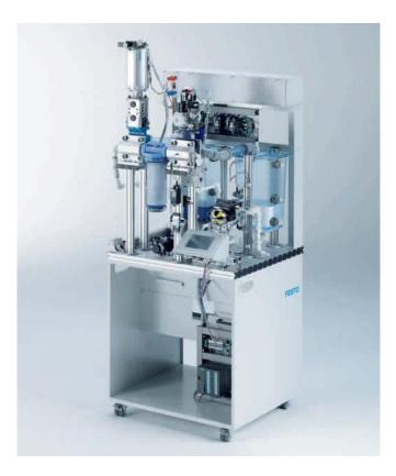
Every MPS® PA station comes completely assembled and tested on the profile plate with MPS® PA trolley, touch panel and 24 V power pack.
