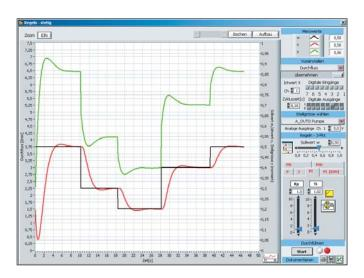
Using FluidLab®-PA step by step to teach and demonstrate the fundamentals of control technology. The EasyPort is used to connect the PC and real hardware, e.g. the EduKit PA, the MPS® PA compact workstation or the MPS® PA filtration station, mixing, reactor, filling.
