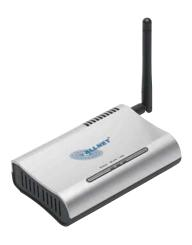
This external access point supports the W-LAN standard IEEE 802.11g with a transmission rate of up to 54 Mbps
