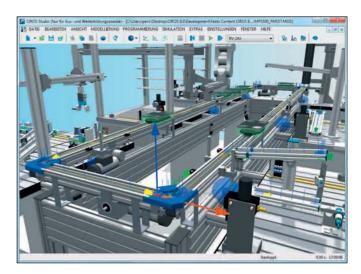
CIROS® Studio is the professional tool for creating simulation models. The industrially utilised, powerful development platform unites the three tools Simulation, Modelling and Programming under one common interface.
