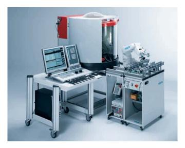
MILL 55 is a 3-axis milling machine of industry-compatible design that facilitates all machining possibilities of a modern CNC milling machine: milling, cutting and drilling/boring.
