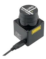
The laser scanner for Robotino® allows the creation of maps, localisation and navigation, as well as obstacle recognition, thanks to the digital detection of objects on one plane. In order to prevent collisions, the 2D laser scanner Hokuyo URG-04LX-UG01 can be mounted above the controller, for an all-round view, or in the loading bay of the Robotino®. The scanner is connected to the control unit and supplied with power via a USB connection.
