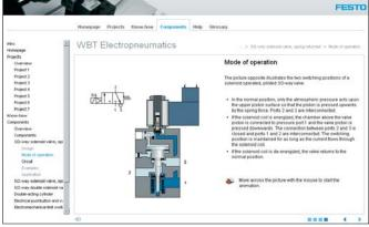
The Electropneumatics training program builds on the Pneumatics training program and reinforces material already learned from practical projects. Starting with concrete industrial applications, fundamental electropneumatic circuits are produced. With the help of numerous exercises, learnt material will be revised, applied and further developed by you. During an exercise, the programme reacts to each answer with varying feedback.
