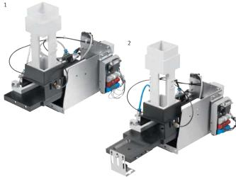
The Conveyor module is intended for mounting on a profile plate, profile foot or slotted mounting frame with freely positionable DC motor. It is suitable for transporting and separating workpieces with a diameter of 40 mm (e.g. "Cylinder bodies" or "Cylinder for assembly" workpiece sets). The module is supplied completely assembled.
