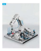
Robot station with MPS® modules
