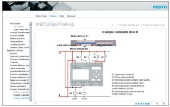
This training program provides an introduction to logic functions. First of all, AND & OR functions and their processing are shown in function tables. Other basic control functions such as memory, timer and counter functions round off the contents. The second part starts by covering the basics of open-and closed-loop control circuits and describes the elements of a controller. It then takes a detailed look at minicontrollers with their features and areas of application.
