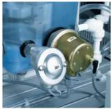
With a P, PI or PID control algorithm, (closed-loop) control technology is taught in a demonstrative and practical manner. The **temperature** sensor – for the Reactor station a PT100 resistance thermometer is used – delivers a uniform signal of 0 – 10 V via the measuring transducer. By way of the continuously controllable heater the controller sets the nominal temperatures and keeps them constant.
