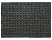
Allows students to determine and compare the losses in a smooth flow channel with those experienced in a channel with a roughened surface.
