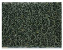
A roughened bed section to allow students to determine and compare the losses in a smooth flow channel with those experienced in a channel with a roughened surface.
