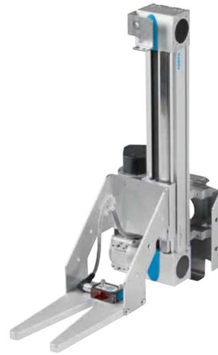
With the easy to use forklift, the Robotino® operates, for example, as a driverless transport system in a production environment.
