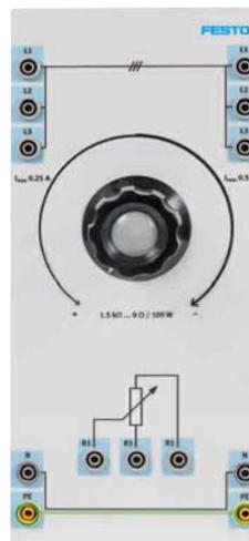
The field rheostat allows the field voltage of motors and generators to be reduced if a set direct voltage is used. By connecting a variable resistor upstream, an exciter field can be set.
