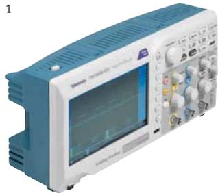
**1 Tektronix TBS1052B-EDU digital storage oscilloscope**
