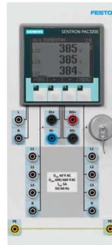
The measurement board is designed for measuring the electrical variables of voltage, current, apparent, real and reactive power, power factor and frequency of one- and three-phase loads. Other functions include min-max values, real and reactive energy, dual tariff recording, average power demand MIN/MAX, hours-run meter and energy meter.
