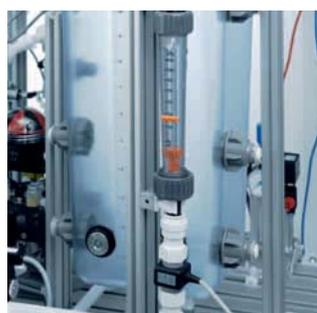
At a constant **flow rate**, the three input materials are mixed into a recipe on the Mixing station. The flow rate is recorded by an electronic flow sensor with an impeller, and is additionally displayed with a float-type flow meter. The controller sets the required flow rate by way of the analogue controlled pump.
