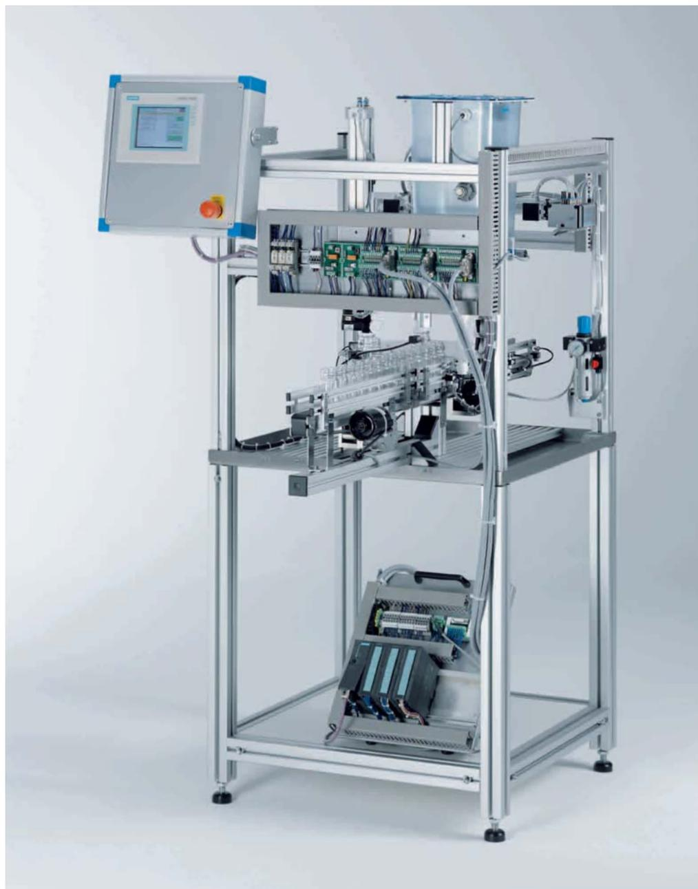
The filling station includes a large number of functions typical to the food industry: Bottle feed by conveyor, dosing with a dosing cylinder and filling and capping on a rotary indexing table.
