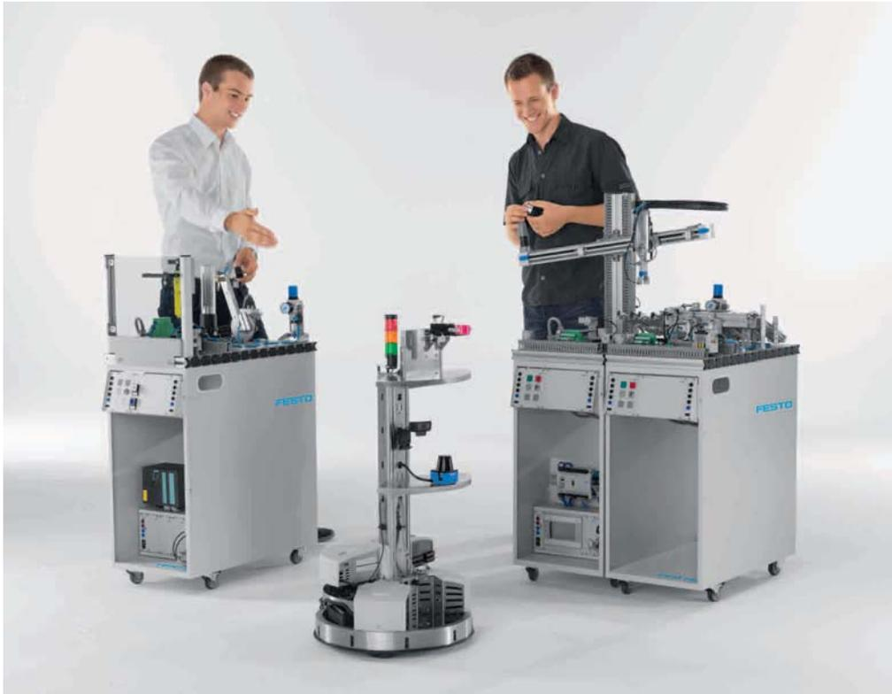
With Robotino®, you can implement your own applications in the fields of mobile robotics and service robotics. The mounting tower allows you to attach standard components or extensions developed by you to Robotino® at any height and to connect them to the control system via the provided interfaces. This means you can convert Robotino® quickly and easily from a forklift truck to a service robot, for example.
