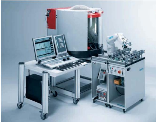
MILL 55 is a 3-axis milling machine of industry-compatible design that facilitates all machining possibilities of a modern CNC milling machine: milling, cutting and drilling/boring.
