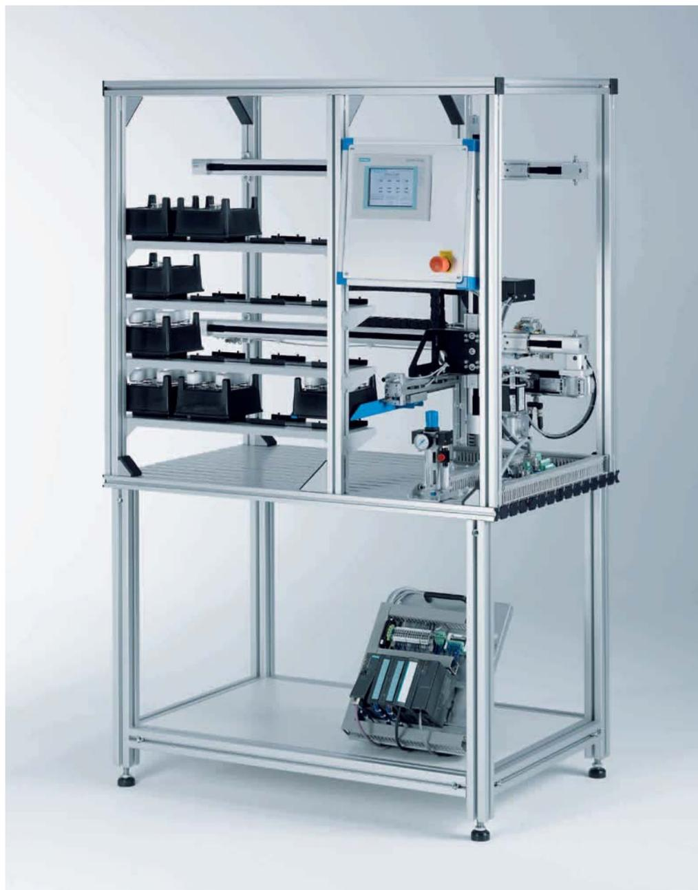
The automatic warehouse can hold up to 16 six-packs on 4 levels each with 4 bays. A cartesian 3-axis handling system is used for stock movement. 2 toothed belt axes are driven by intelligent servomotors with an integrated servo amplifier, controller and CAN bus interface.
