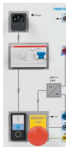
The supply unit ensures safe operation of single-phase servo controllers or frequency converters at workstations where there is no corresponding infrastructure. It is connected to the mains supply via a non-heating device cable and makes it possible to provide an electrically safe workstation even in places where there is no separate fuse protection or type B RCD protection available.
