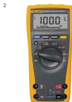
**2 Fluke 179 digital multimeter**
