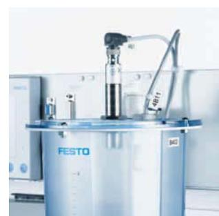
In the Filling station the **level** of the dosing tank is recorded with an analogue level sensor. By way of the continuously controllable pump the controller regulates the level to the appropriate nominal value. During filling, the level in the dosing tank is kept constant, thereby optimising the filling quality.
