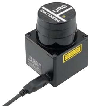
The laser scanner for Robotino® allows the creation of maps, localisation and navigation, as well as obstacle recognition, thanks to the digital detection of objects on one plane. In order to prevent collisions, the 2D laser scanner Hokuyo URG-04LX-UG01 can be mounted above the controller, for an all-round view, or in the loading bay of the Robotino®. The scanner is connected to the control unit and supplied with power via a USB connection.
