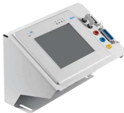
Touch screen for flexibly displaying processes and data with integrated Codesys® PLC for open and closed-loop control of processes in accordance with IEC 61131. 8 digital inputs and 8 digital outputs can be used via SysLink. The Sub-D 15-pin connection is designed for 4 analogue inputs and 2 analogue outputs. 4 mm safety sockets are available for emergency stop and external power supply.
