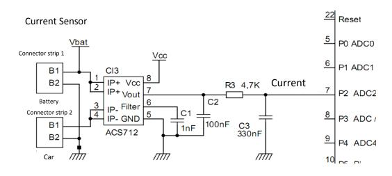
The current emitted by the + connector of the battery travels through pins 1 and 2 towards pins 3 and 4.
