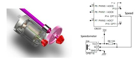
The sensor used here is a reflection detector. An infrared light is emitted by a diode and is then reflected by the white stripes and not the black ones. The signal transmitted to the sensor is sent to a counting input on the microcontroller, and the counter increases at each change of state from white to black or black to white. Each incremental change of the counter corresponds to a travelled distance that remains to be calculated. The coder has 6 white stripes and 6 black stripes.
