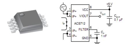
The resolution of the circuit is of 100mv/A. The measurement range goes from -20A to +20A. Here, only positive currents are measured.
