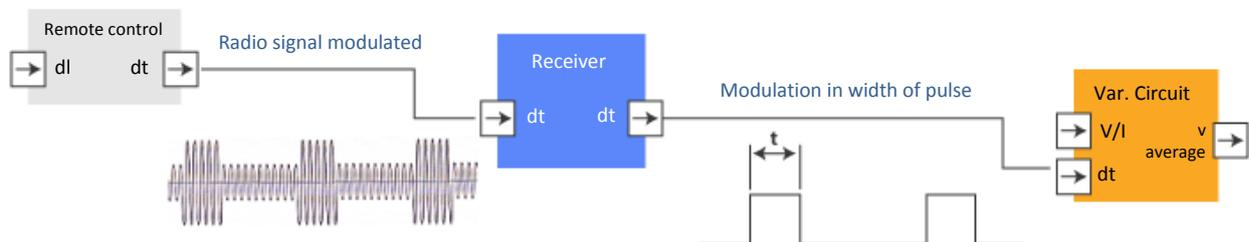
We will now measure the command signal on the receiver to describe it entirely. At the output of the receiver, we find two channels with red, black and white threads. One is for the controller, and the other is for steering.
