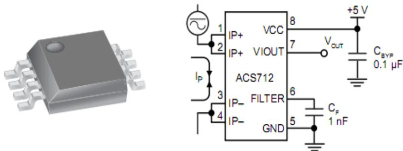
The resolution of the circuit is of 100mV/A. The measurement range goes from -20A to +20A. Here, only positive currents are measured.
