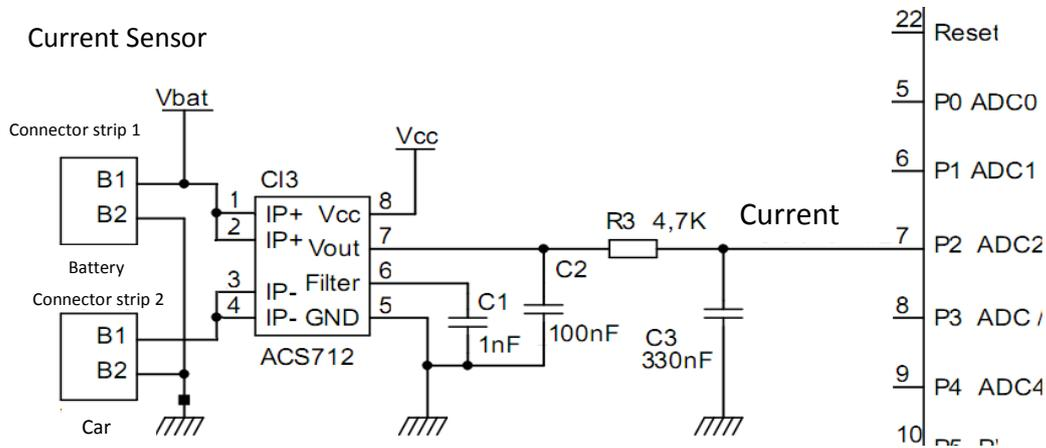
The current emitted by the + connector of the battery travels through pins 1 and 2 towards pins 3 and 4.
