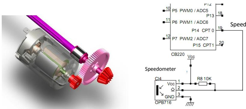
The sensor used here is a reflection detector. An infrared light is emitted by a diode and is then reflected by the white stripes and not the black ones. The signal transmitted to the sensor is sent to a counting input on the microcontroller, and the counter increases at each change of state from white to black or black to white. Each incremental change of the counter corresponds to a travelled distance that remains to be calculated. The coder has 6 white stripes and 6 black stripes.
