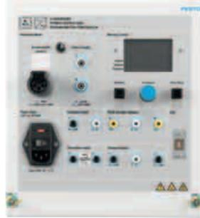
**Four-Quadrant Power Supply and Dynamometer Controller**
