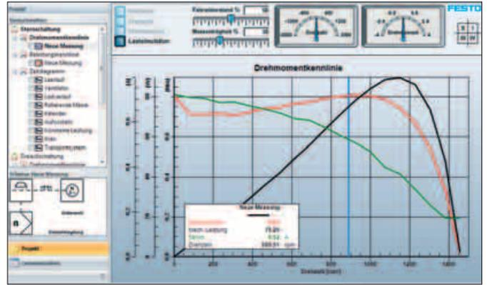
The convenient and intuitive **Drive-Lab** software supports the automatic recording of machine characteristic curves, the parameterisation of a static load and the simulation of load models for the examination of drives under realistic conditions. The comparison and optimisation of different drive concepts can be carried out in the form of project exercises. Sample configurations provide a quick and easy-to-understand introduction.
