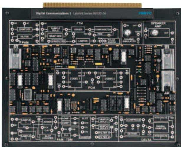
The Digital Communications 1 course provides comprehensive, hands-on instruction in the terminology, principles, and applications of digital circuits, including: Sampler, Sample/ Hold, Adder, Ramp Generator, Comparator, Limiter, Filter, CODEC, PLL, Compressor, Expander, Integrator, Differentiator, Latched Comparator, Speaker Amplifier, and Channel Simulator.
