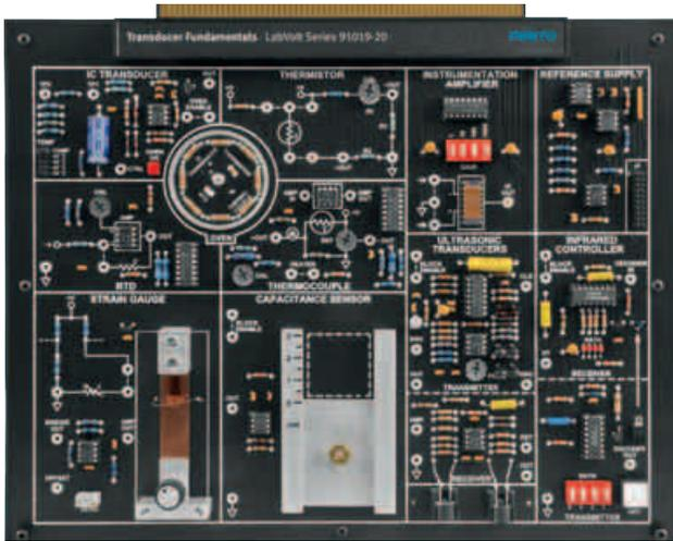
The Transducer Fundamentals course guides students through the circuits and devices used to interface computer and control circuits. Students learn the principles of input and output transducers and how physical quantities, such as heat, position, proximity, and force, are converted to electrical signals for detection and processing.
