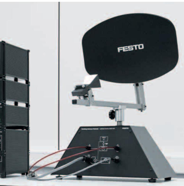
Communications and radar training systems from Festo Didactic incorporate hands-on experience with the principles and operations of electronic communications and radar systems.
