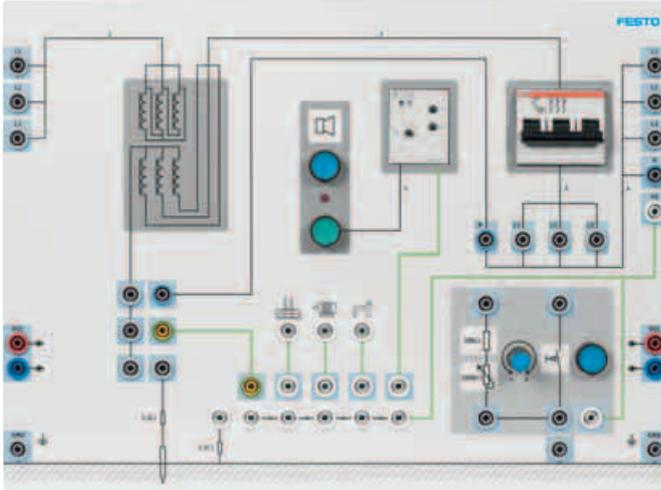
The IT network EduTrainer® expands the equipment set for mains systems and protective measures to include the topic of IT systems. The integrated fault simulator allows simulation of insulation faults which are detected and displayed by the insulation monitor. If the adjustable value is fallen short of, this is indicated by a lamp, as well as a buzzer which can be acknowledged.
