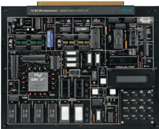
This board provides comprehensive, hands-on instruction in the terminology, principles and applications of 32-bit  $\mu$ C microprocessor systems.
