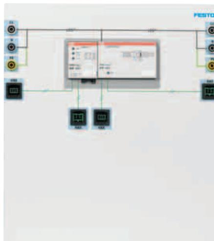
The line connector connects the main and secondary line in a KNX systems. This also permits targeted filtering of signals. The main line is also equipped with a power supply. The plate also contains the KNX system distributor for 230 V.
