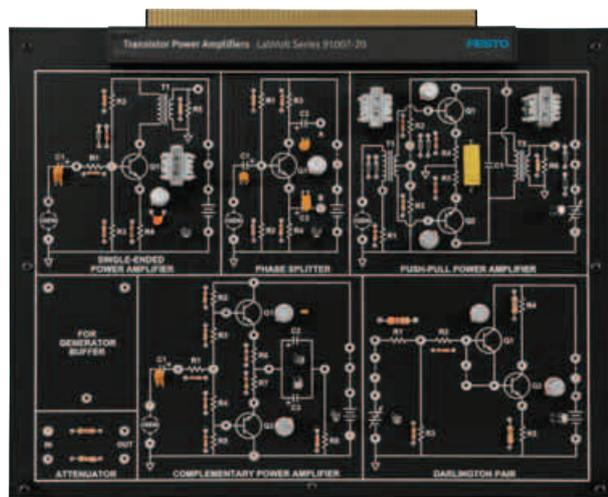
The Transistor Power Amplifiers Circuit Board is designed to teach troubleshooting of transistor power amplifier circuitry.
