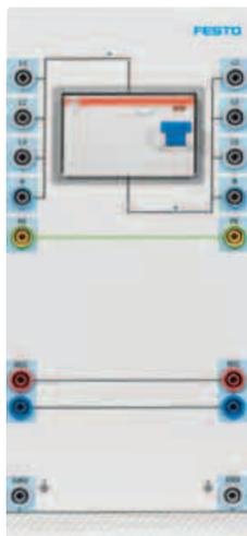
The Selective RCD EduTrainer® allows for treatment of the topic of selectivity for residual current circuit breakers in mains systems and protective measures. The selective RCCB ideally supplements the RCD A/B EduTrainer®, so that it can be easily integrated and its essential characteristics can be elaborated.
