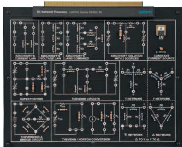
Consisting of nine training circuit blocks and a constant-source current block, the DC Network Theorems Circuit Board enables students to perform practical exercises that demonstrate theoretical DC principles. When a circuit has two voltage sources in different branches, theorems are used to solve for voltage and/or current in these circuits where Ohm's Law cannot be applied.
