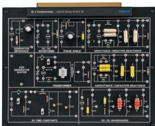
This Circuit Board contains nine circuit blocks on which students perform varied troubleshooting exercises in the AC 1 Fundamentals program. Students identify and isolate the following circuits: Generator Impedance, AC/DC Waveforms, Phase Angle, Inductance/Inductive Reactance, Transformer, Capacitance/Capacitive Reactance, RC Time Constants, and RC/RL Wave Shapes.
