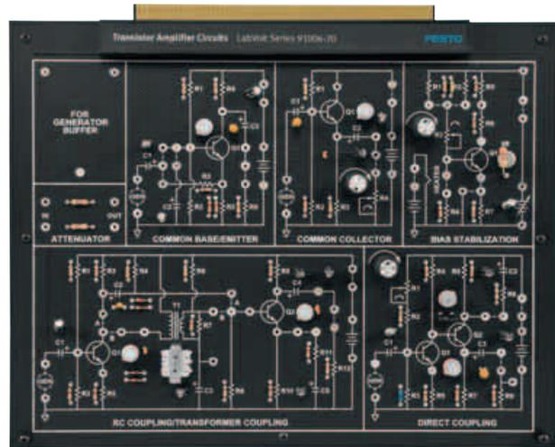
The Transistor Amplifier Circuits Board allows students to perform practical exercises that demonstrate transistor amplifier principles.
