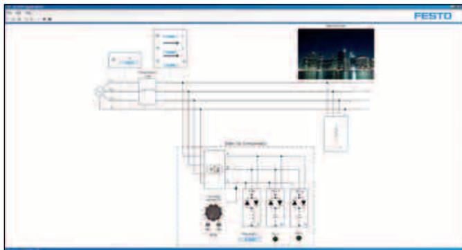
SCADA for LVDAC-EMS is a software program designed to run in combination with LVDAC-EMS. It transforms LVDAC-EMS software and the workstation's computer into a local workstation that can be monitored and controlled over a local network from a supervisory computer.
