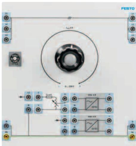
Single-phase variable transformer for providing a variable alternating current.
