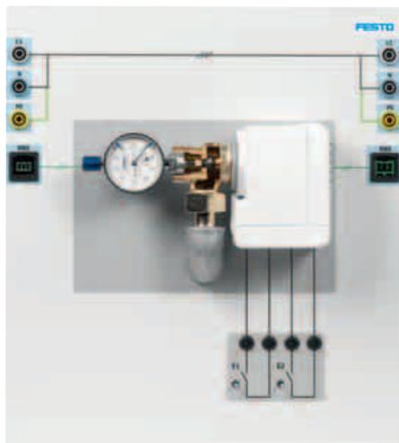
The heating actuator controls the heating water circuits in heating systems. The interior of the valve is visible, and an integrated gauge shows the stroke of the plunger. The valve is supplied entirely via the KNX bus. Two binary inputs are available as presence and/or window contacts and can be controlled via switches or external signals. The plate also contains the KNX system distributor for 230 V.
