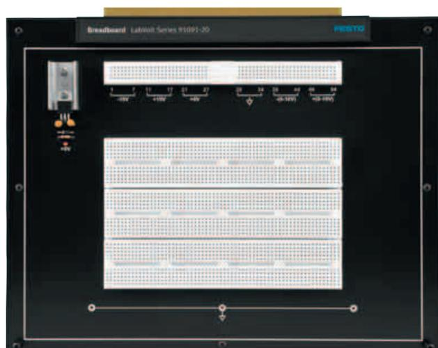
The Breadboard is a complement to Digital Logic Fundamentals (Model 91014). The Breadboard module consists of three printed circuit boards designed so that students can easily connect and change circuits without the need to solder components.
