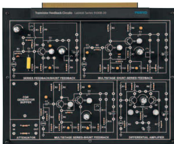
The Transistor Feedback Circuit Board enables students to perform practical exercises that demonstrate Transistor Feedback principles.
