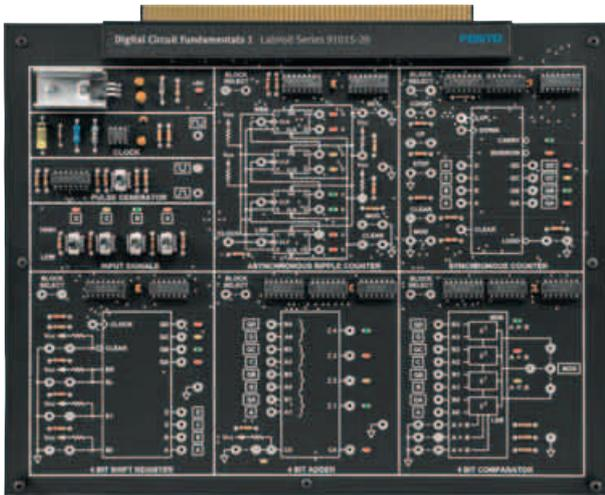
The Digital Circuit Fundamentals 1 course provides comprehensive, hands-on instruction in the terminology, principles, and applications of digital circuits.
