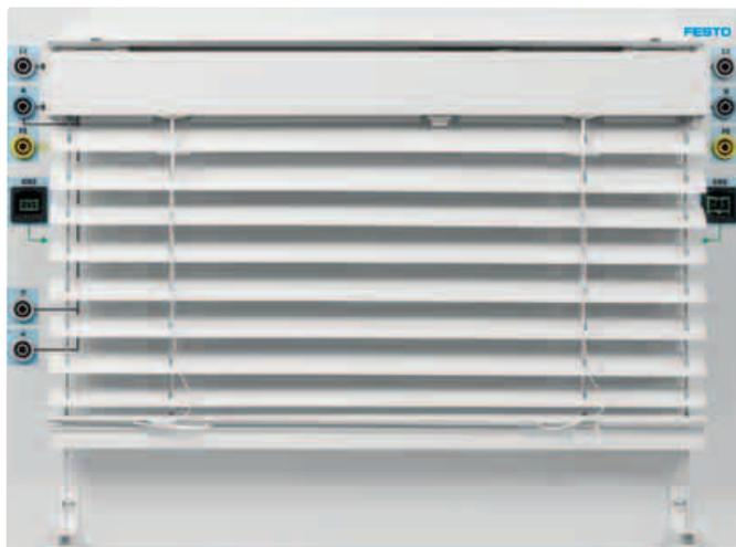
The louvre is used to emulate situations in building automation. For this purpose, the louvre can be raised or lowered and the slat position can be influenced. The connections for controlling “UP” and “DOWN” are routed to 4 mm safety sockets. The plate also contains the KNX system distributor for 230 V.
