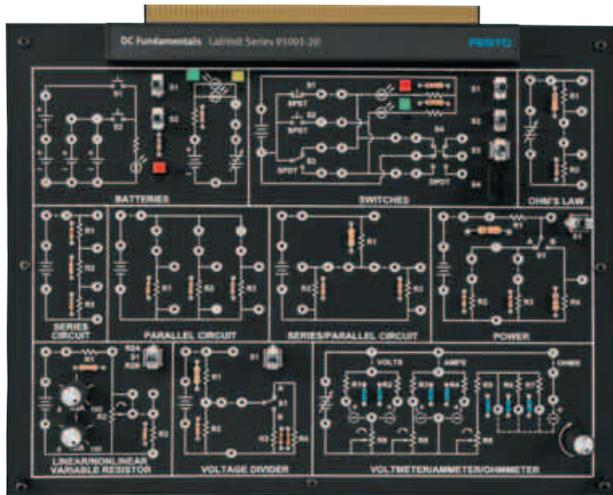
The DC Fundamentals Training Circuit Board is used by students to perform practical exercises that demonstrate DC principles. Students will become familiar with all the components to be able to successfully identify and isolate the circuit blocks on the training board and perform trouble-shooting exercises.
