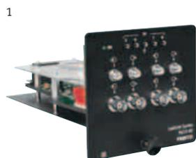
**1 Radar target tracking interface**
