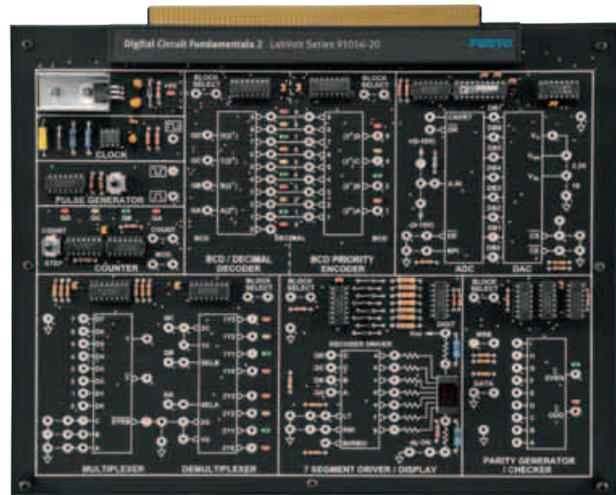
The Digital Circuit Fundamentals 2 course provides comprehensive, hands-on instruction in the terminology, principles, and applications of digital circuits.
