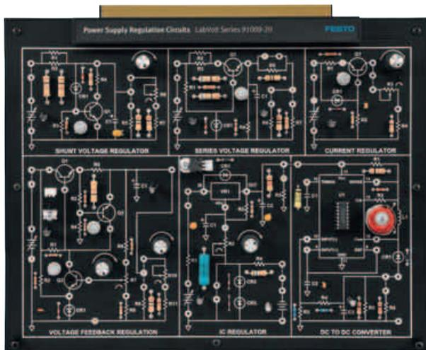
The Power Supply Regulation Circuits Board provides comprehensive, hands-on instruction in the terminology, principles, and applications of power supply regulation circuits.
