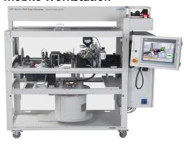
The mobile workstation consists of a sturdy, welded-steel frame painted using powder-coated paint for a durable surface. The unit is mounted on four swivel casters with a locking mechanism that allow easy motion and stable operation.
