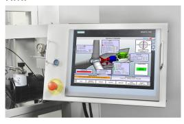
The nacelle controller consists of a touch-screen panel that runs the human-machine interface (HMI) connected to the PLC used to command and monitor the system. The interface is available in English, French, German, and Spanish.
