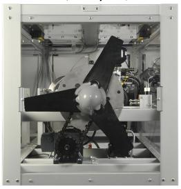
The entire drive train is driven by a 560 W (3/4 hp) gear motor just beside the yaw mechanism. This motor drives the nacelle main shaft and blades (with a fixed pitch) through a chain. The main shaft passes through two pillow blocks and then into the gearbox. The main shaft also includes a rotor-lock mechanism and a speed sensor. The main shaft is attached to the gearbox with a shrink disc similar to that which can be seen in an actual nacelle.
