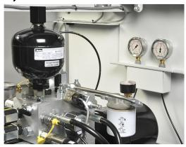
The training system includes a custom hydraulic unit which controls the two hydraulic brakes in the system.
