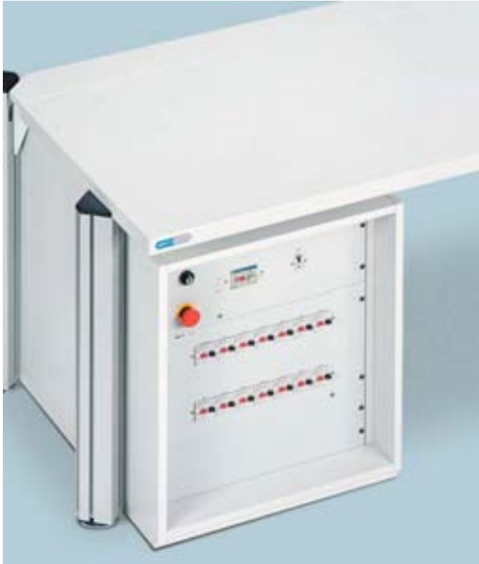
19 inch drawer unit, floor-mounted, of a system width of 525 mm, usable front height 13 HE/19inchl; 1 HE = 44.45 mm. The 19 inch suspended drawer unit is suitable for the installation of devices of the 19 inch technology. Sturdy sliding rails can be built inside the cabinet for deep devices. The 19 inch containers are particularly suited for the installation of partitionings in teacher's working places in training centres. On request the 19 inch baseom cabinet can be equipped with a front door.
