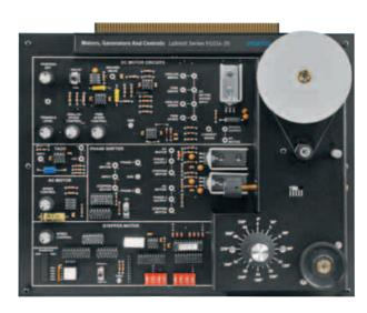
The Motors, Generators, and Controls course provides comprehensive, hands-on instruction in the terminology, principles, and applications of the DC motor, AC synchronous motor, phase shifter, and stepper motor.
