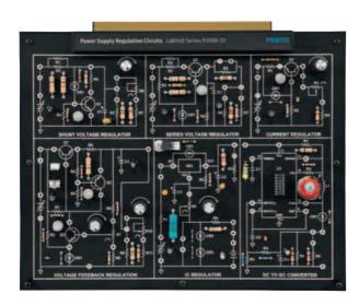
The Power Supply Regulation Circuits Board provides comprehensive, hands-on instruction in the terminology, principles, and applications of power supply regulation circuits.
