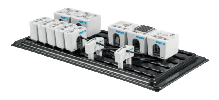
Extend the study of fundamental electrical engineering and electronics to opto-electronics The training package Opto-electronics expands on TP 1011 or TP 1011M to provide a comprehensive introduction to optical electronics. The kit enables students to explore the combined use of electronics and light. They will learn about optical semiconductor behavior, construction, and characteristics.
