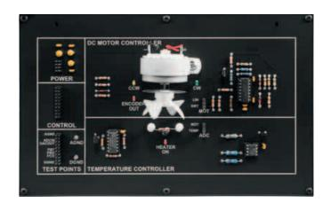
This Circuit Board is an add-on to the 32-Bit Microprocessor (Model 91017). It allows students to study how microprocessors can control and communicate with external devices. The Application Board has two application circuits: a DC Motor Controller, and a Temperature Controller.
