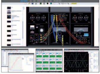
Electromechanical Systems Simulation Software (LVSIM®-EMS) is a simulation software that enables students to perform actual experiments using virtual equipment
