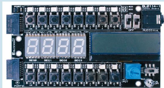
Note: This tutorial refers to the port settings (ports A and B) as used with PIC. For Arduino users, please use ports C and D as appropriate. (Port C on the Arduino 'Maps' to Port A of the Combo board).
